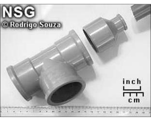
Materials: (1) a 2" or 3" T-joint; (2) a 2" or 3"  $\times$  1" coupling; (3) about 3' of 1" pipe for the handle; (4) PVC glue/cement.
